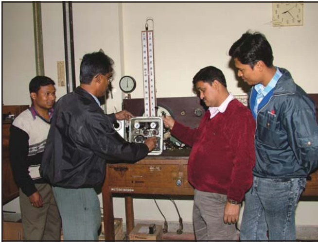
Instrumentation personnel servicing a pneumatic instrument
